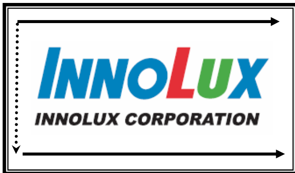
Fig. 1 Normal scan ( pin 4, LR/UD = High or NC )
