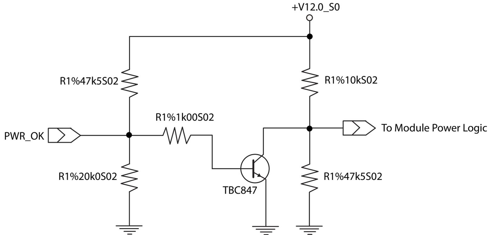
The voltage divider ensures that the input complies with 3.3 V CMOS characteristic and also makes it possible to use the module on carrier board designs that do not drive the PWR\_OK signal. Although the PWR\_OK input is not mandatory for the onboard power-up sequencing, it is strongly recommended that the carrier board hardware drives the signal low until it is safe to let the module boot-up.
