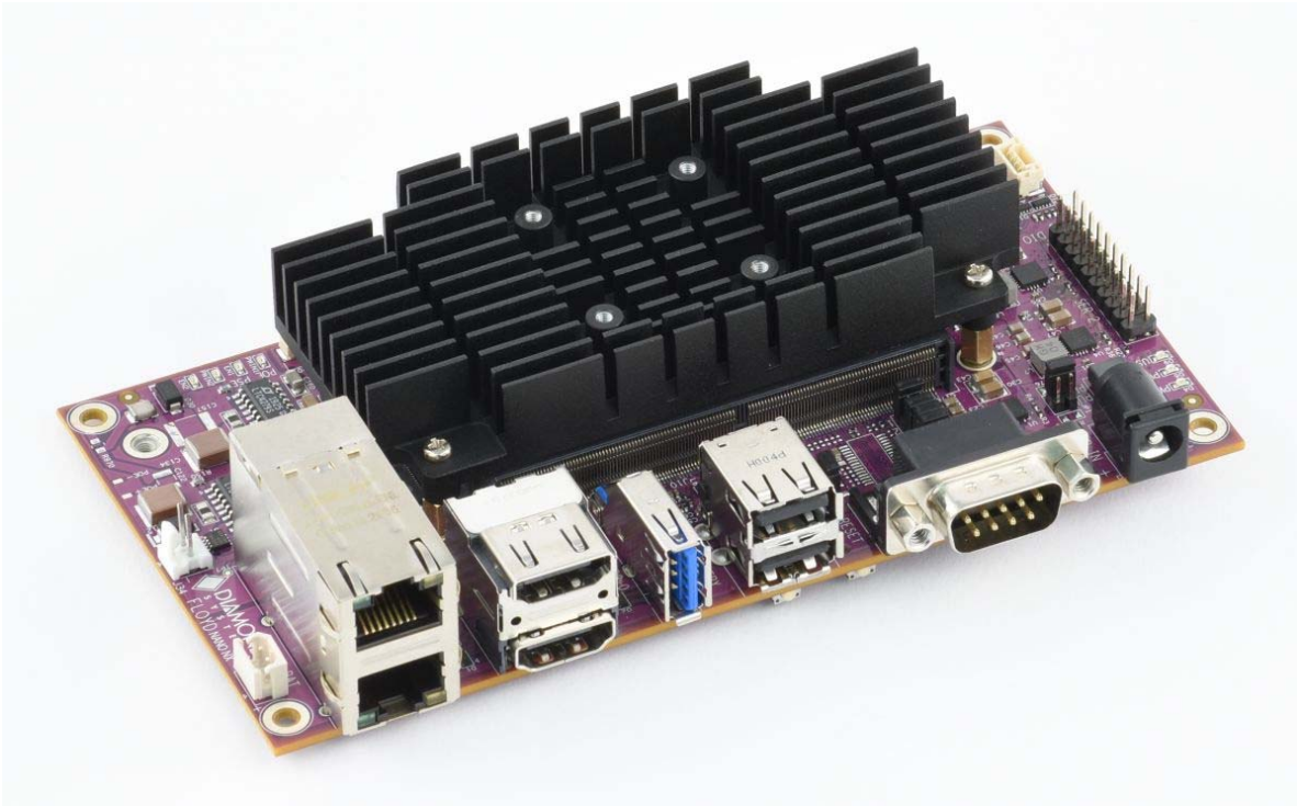
Figure 12-2: Floyd with Heat Sink Installed
