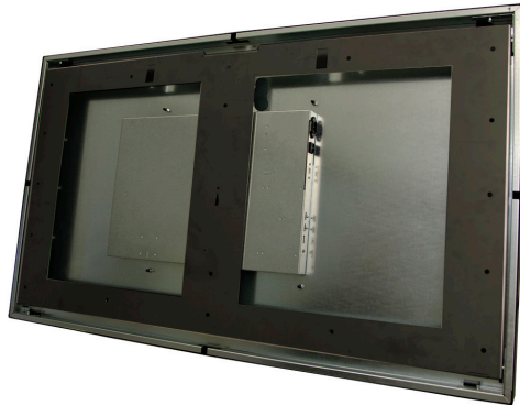
BLO-Line® 4K 42.5 monitor backside incl. wall mount (darker coloured for demonstration)
