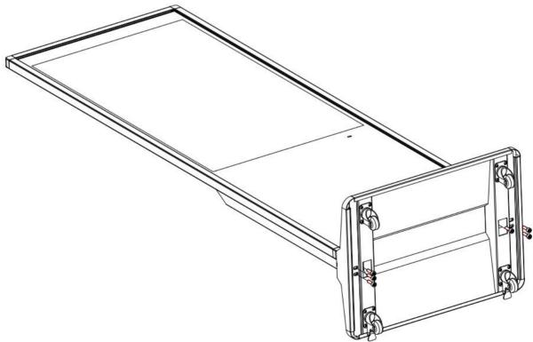
Insert the corresponding gap of the machine and fix the M8 hexagon socket head screw
