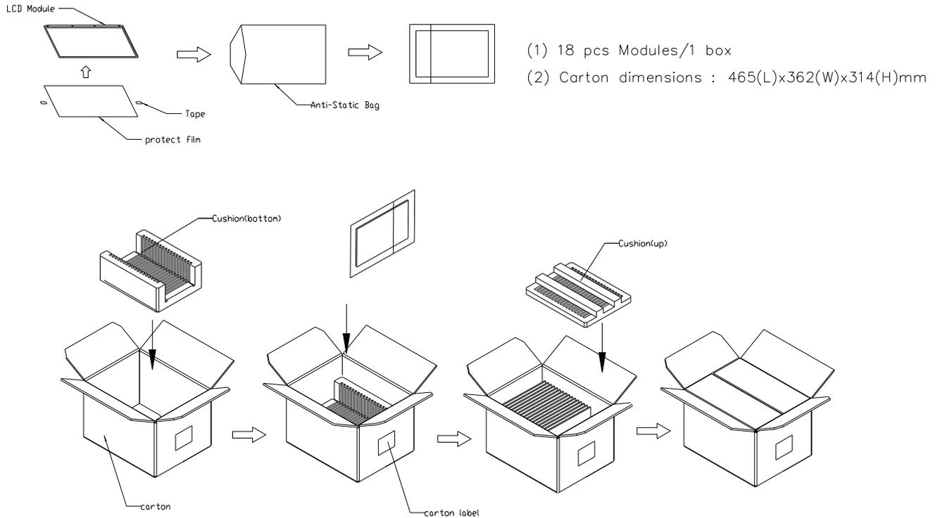
**Figure. 9-1 Packing method**
