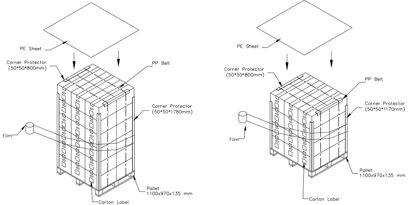
**Figure. 9-2 Packing method**
