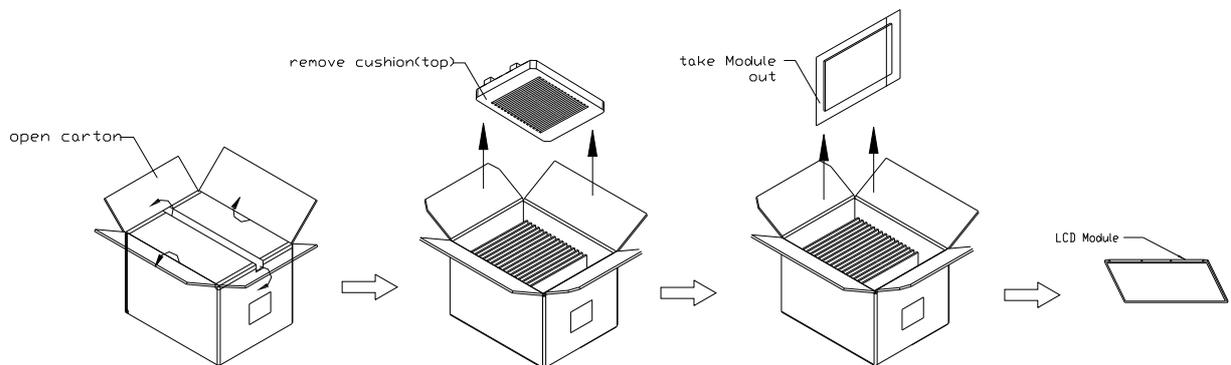
**Figure. 9-3 UN-Packing method**
