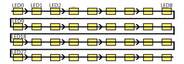
LED0 is in the upper left corner of the screen. LEDs increment left to right and continue incrementing on the left LED of the row below.
