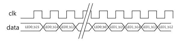
Data is to be transmitted on the rising edge of CLK MSB first starting at LED0; see scan direction reference below. Data much be transmitted for all LEDs for the panel to update brightness. To reject data prior to completing transmission, resend the start transmission condition.
