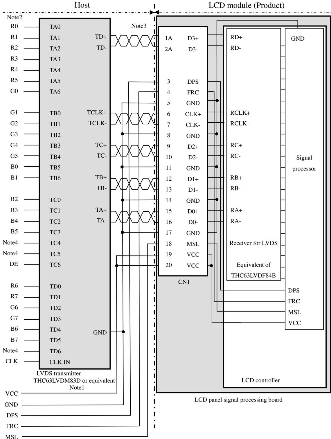
Note1: Recommended transmitter: THC63LVDM83D (THine Electronics Inc.) or equivalent
