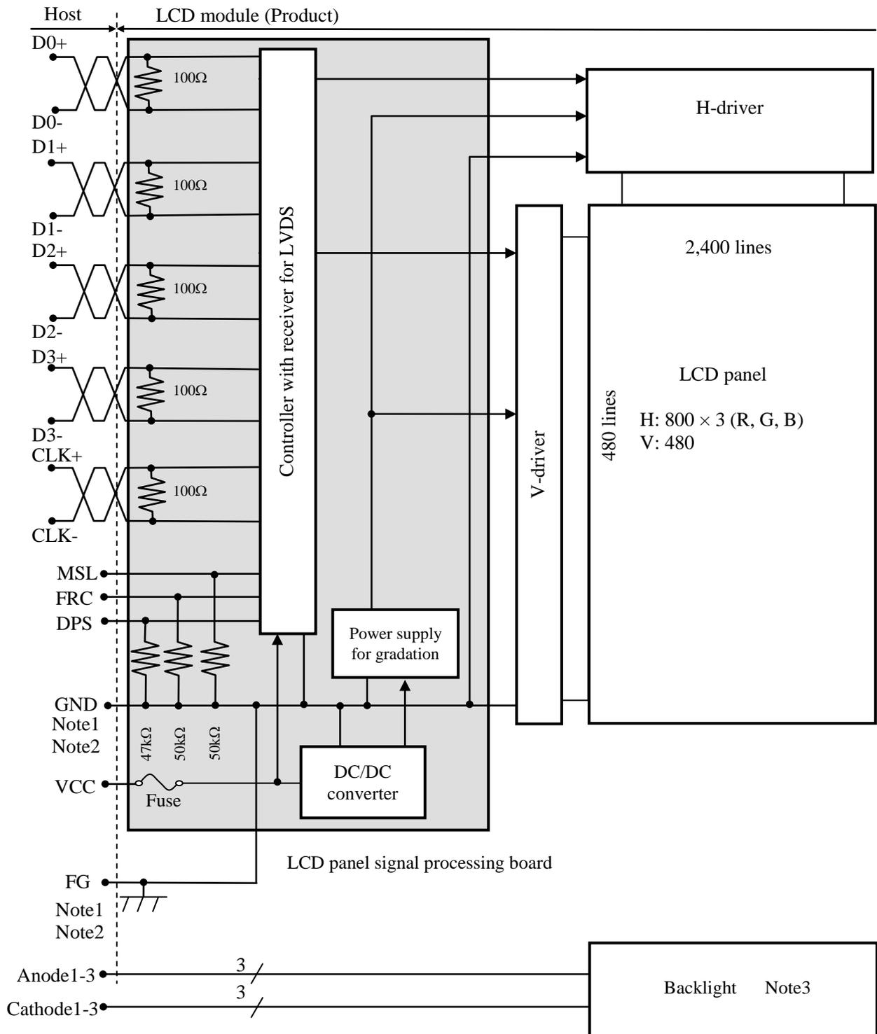
Note1: Relation between GND (Signal ground) and FG (Frame ground) in the LCD module is as follows.
